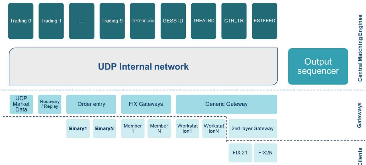
The previous diagram shows the different layers of processes. Client applications establish connections to one of the Gateways. For instance, a client application “Binary 1” can establish a connection with the Order Entry Server.
